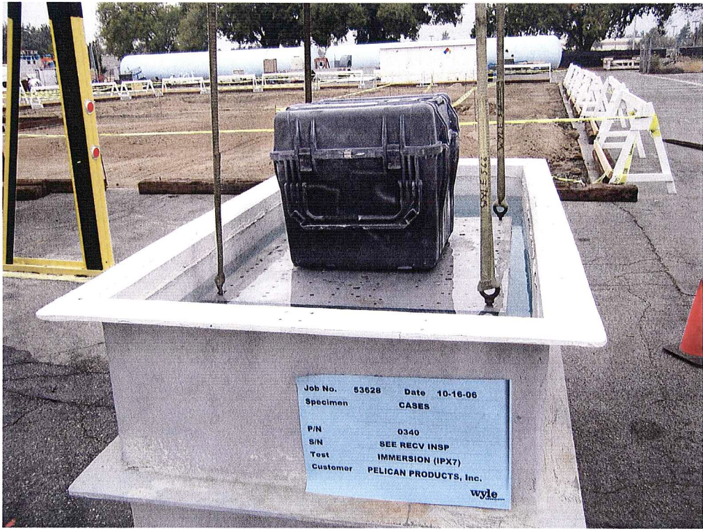
Photograph 4 Immersion Test Setup
