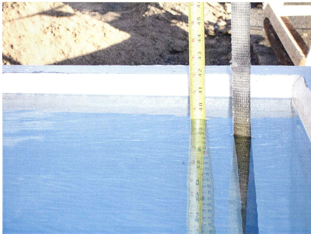
Photograph 6 Immersion Test Setup
